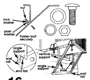
**TO** Secure vertical and angle supports together. Attach supports to bottom of cabinet. <u>But Do Not tighten</u> bolts at this time. Attach wall rail to angle supports. Slide each support assembly toward house until wall rail is positioned firmly against wall. Note: If your house is constructed of material that could be damaged by wall-mounting support, fasten a board between wall rail and house.
